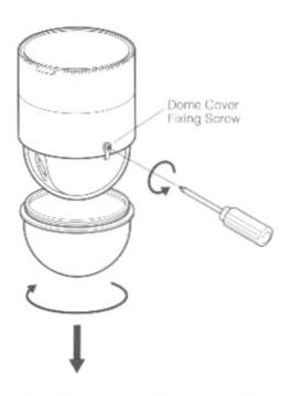
Remove the Domo Cover of the WV-CS604 or WV-CS404 by turning it counterclockwise.
