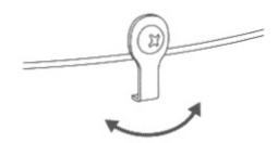
Attach the WV-CS1S Dome Cover to the camera by turning it clockwise.
