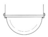
Fix the WV-CS1S Dome Cover by fixing the two Dome Cover Fixing Screws removed just before.
